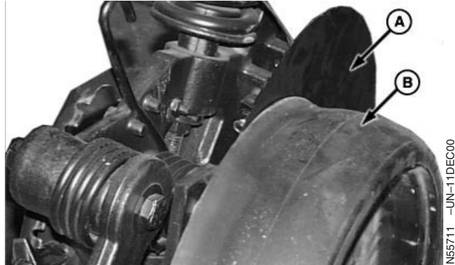
A—Disk Opener B—Gauge Wheel
