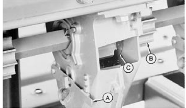
A—Latch B—Feed Roll C—Seed Retainer Ring
